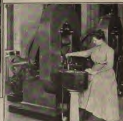
3. Making the disks into gold eagles by stamp- ing them with the steel dies.
